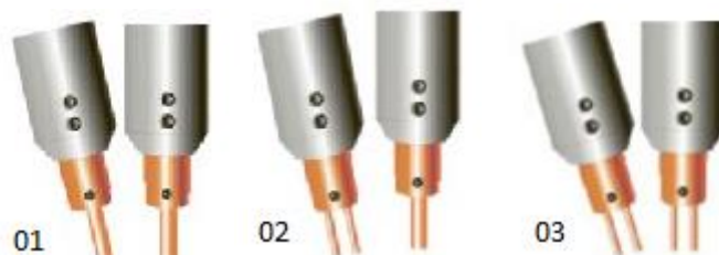
Figura 20 - Esquema de soldagem SAW tandem wire . 01 – Single + single; 02 – Single twin ; 03 – Twin + twin .
